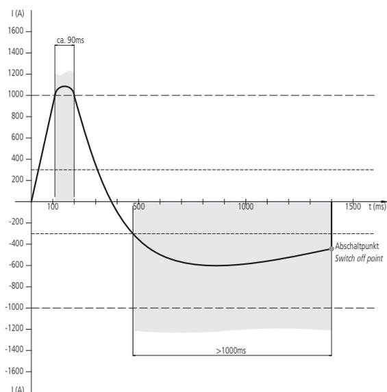
The electronic measures the main current galvanically isolated and switch-OFF the relay whenever the threshold is exceeded. The relay remains switch-OFF until again reset by switching-OFF-ON INIT or switching-ON-OFF the supply voltage.
