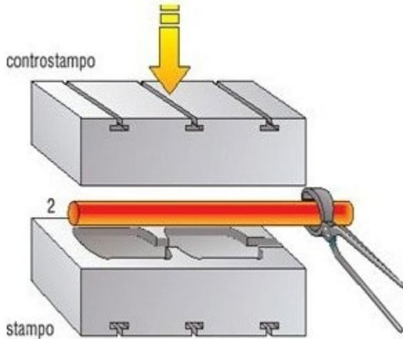
*Die-Casting and hot forging are the most commonly used processes for manufacturing battery terminals.*
